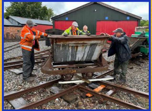
The permanent way team demonstrate how to turn a skip at a right angle, using a portable point (probably not its proper name).
